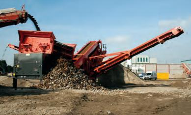
At the heart of the QA451 is the Triple deck Doublescreen box, featuring two independent triple deck screen boxes. Both feature independent drives and can have their amplitudes and combined screen angles adjusted dependant upon application. The QA451 offers a screening solution no other mobile triple deck screener can provide as its two screen boxes offer an unsurpassed level of separation on a wide range of materials, at very high rates of production.
